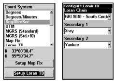
Setup Loran TD highlighted on Coordinate System menu (left). Configure Loran TD menu (right).
